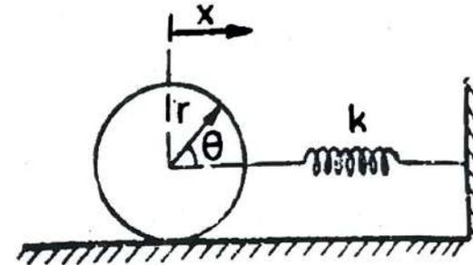
Determine the frequency of horizontal oscillations of the system if the cylinder :
